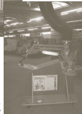
Suction cup gripper - Saint Hilaire woodwork unit
